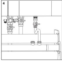
1-2. Keep the cap on the connections that are not used on the pipe work headers:
