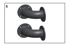
The pipe work headers are available in 2 dimensions, i.e. DN65 and DN100 and are connected to one another by the flange couplings and gaskets, M12 or M16x55 bolts, spring washers and nuts. The low loss header and the complete installation can then be connected to it.
