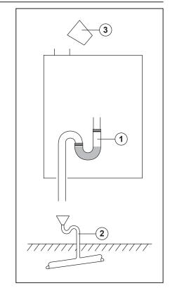
For a cascade system, fit a pipe work header for the condensate drain behind the hydraulic system. For that purpose, the flange plates have holes allowing the installation of a PVC drain of ø40mm max. Use this drain to connect the individual condensate drains of each boiler.
